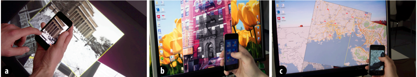
Figure 1. Virtual Projection is inspired by its optical counterpart for transferring information between handhelds and stationary displays such as tabletops, PC displays or large public displays. By fixing the virtual projection to the display, the frustum can also be used to (a) select regions, (b) interactively apply filters, and (c) post multiple views.
